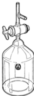
Fig 2: Specialty glassware for storage of pyrophoric materials
